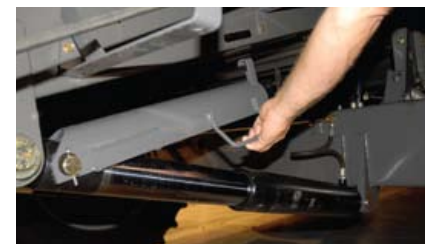
Responsive 3" (76 mm) lift cylinders on the 660B and 670B, and 3.5" (89 mm) lift cylinders on the 680B provide the strength and capacity to quickly lift heavy headers, including the large 35 ft. (10.9 m) FHB Series flex header and the 12-row CH Series corn head.
