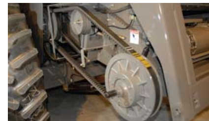
A variable-speed head drive matches the corn head and feed chain speed to ground speed for greater productivity and reduced crop loss. A standard feature on corn/soybean models, it's also optional on grain versions.
