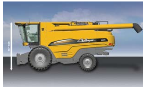
When the grain tank extensions are folded, the 600B series combines measure only 147 in. (3.73 m) in height (with 30.5L32 front tires).
