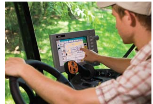
With the press of a button, the operator can move to virtually any display without scrolling through multiple screens. The monitor can also be customized to display the information that is most important to the operator.
