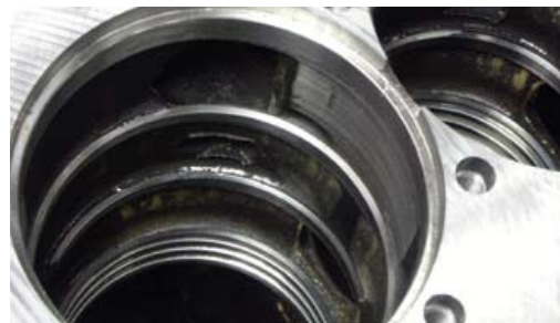
Dual Liner Support: Less vibration and liner cavitation for longer cylinder life.
