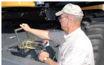
A single-point multi-coupler, which combines all electrical and hydraulic connections into a single one allows for faster and cleaner connections.
