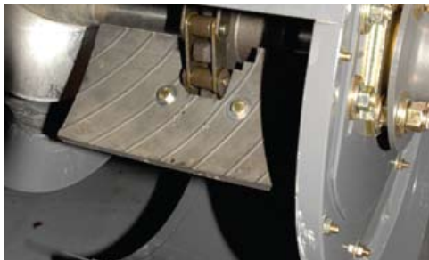
The paddles on the clean-grain and tailings elevators feature bolts, instead of rivets, for easy replacement, should it become necessary.
