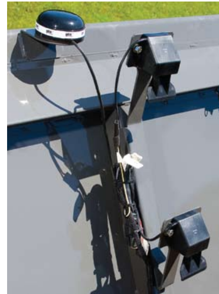
The grain bin "full" sensor, which is also connected to the optional rotary beacon, alerts the operator when the grain tank is 75% full.
