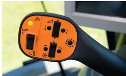
The unloading auger is controlled from the multifunction handle. A switch in the auger prevents engagement if it's not fully extended.
