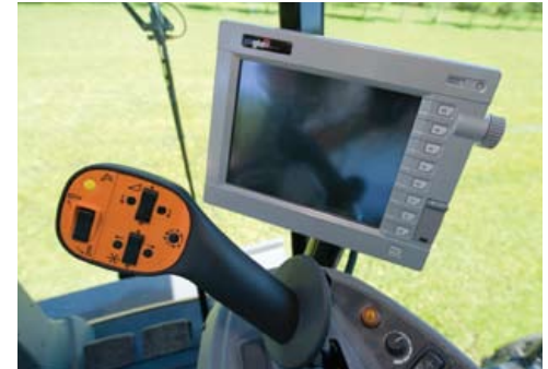
The position of the C2000 terminal can be adjusted independent of the seat-mounted console for easy access to the touchscreen and dials, as well as maximum visibility.
