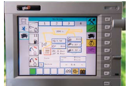
The C2000 terminal displays information in a manner that is most beneficial to the operator. Engine temperature, oil pressure and fuel level, for example, are displayed as analog gauges or they can appear digitally on the screen.
