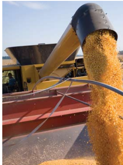
Challenger's "direct flow" unloading auger uses only two augers instead of three for smooth, gentle grain flow. Because grain does not have to change directions during unloading, you'll also experience higher grain quality, less wear and reduced horsepower consumption.
