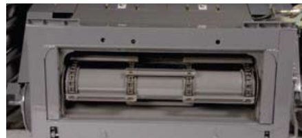
Designed for durability, the feederhouse is equipped with a jaw clutch that protects the system during excessive conditions, while #557 chain with chrome pins provides a longer service life. Chain slats are even bolted on, rather than riveted, for simpler replacement.
