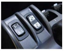
As an added benefit, the system has the unique ability to couple A and B engine speed settings with the ground speed memory system. When activated, this feature allows the operator to alter both the engine speed and the transmission ground speed with the "SV1" and "SV2" buttons.
