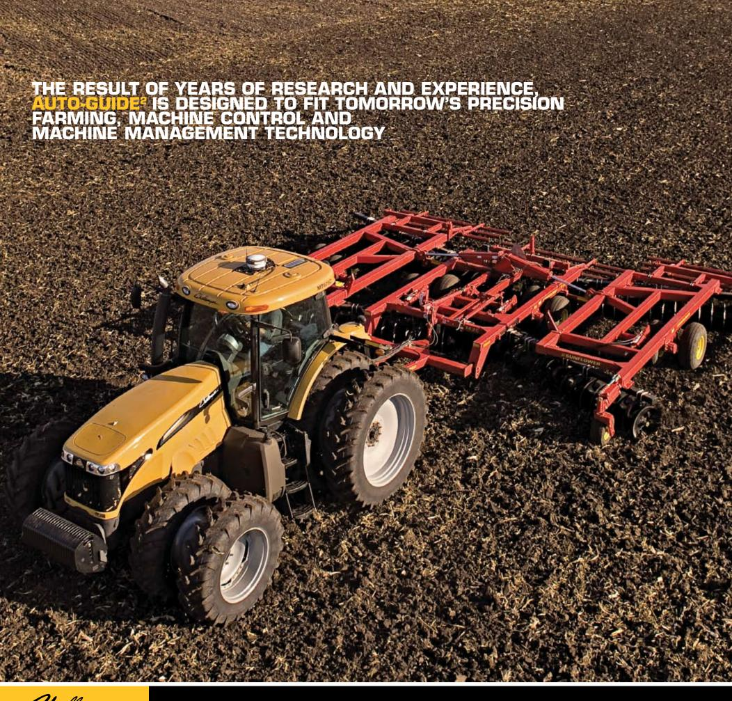
Fortunately, the advanced electronic features on the MT600C allow you to do that. Working in conjunction with the standard radar, the MT600C offers more than 20 valuable monitoring, control and comparative functions, including wheel slip, fuel/hour, distance, cost/hour, area worked, etc.
