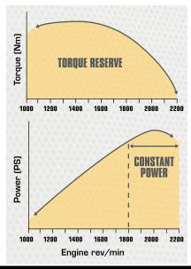
The engine maintains maximum torque between 1,200 and 1,500 rpm and delivers constant power down to 1,570 rpm. A 54% torque bulge on the AGCO SISU POWER engine is more than adequate to pull you through those tough spots in the field.
