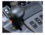
By using both its mechanical and hydraulic capabilities at the same time, the TechStar CVT not only operates more efficiently, but it does so without preset gear limits, providing the operator with speed choices normally hidden in the areas between gears. There's no shifting of gears, no jerks and no delay in traction or power — just infinite speed control from creep to transport speed.
