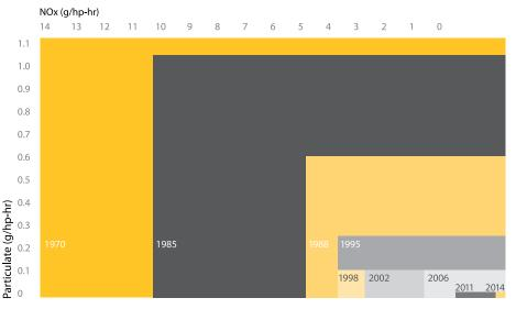
What lies ahead: This chart shows how EPA standards have grown progressively more stringent since the early days of emission regulation. Tier-4 interim requirements go into effect in 2011 and Tier-4 final standards must be met by 2014. At each step, reduced NOx and PM emissions are represented by a smaller rectangle.
